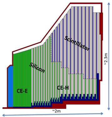
Electromagnetic calorimeter (C**E-E**):
