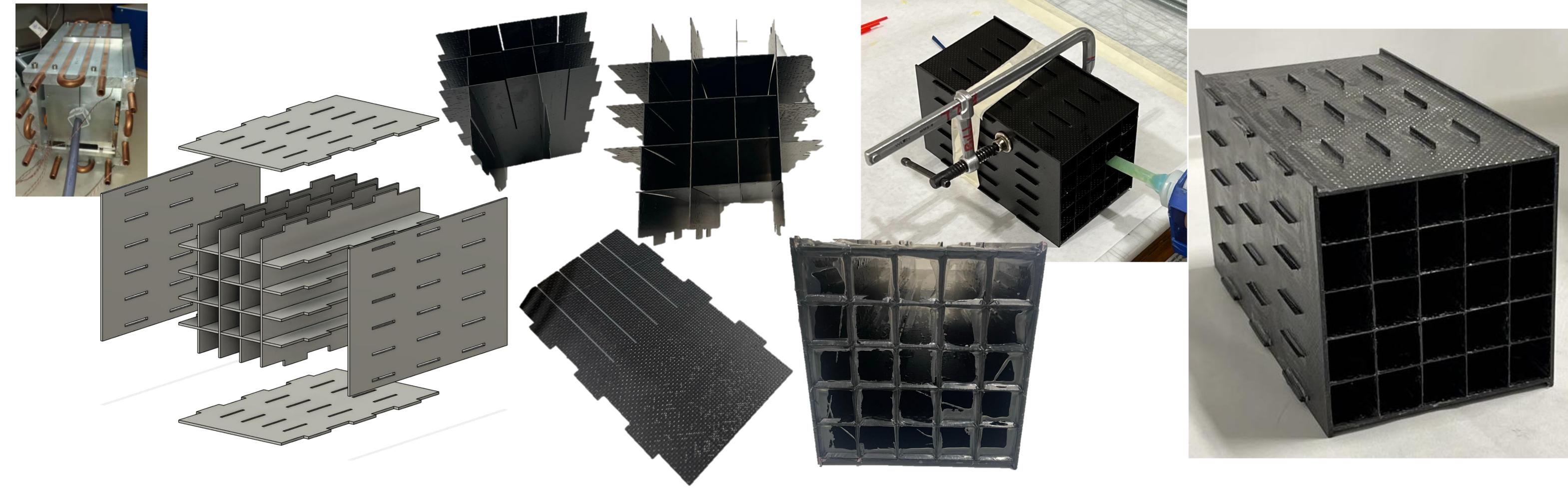
Fig.3. CalVision: carbon fiber composite support structure for calorimeter with integrated cooling
