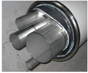
Compound cryogenic distribution line (incl. ScHe supply and VLP return)
