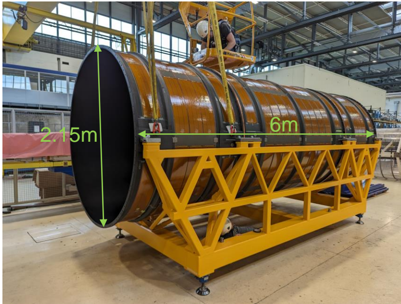
ATLAS ITk Outer Cylinder
