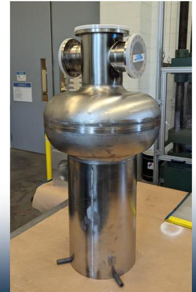
R137mm beampipe stub brazed to a flange
