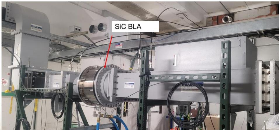
High power test setup with 704MHz 1MW CW klystron Standing wave with short plate
