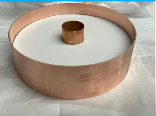
Inner conductor test braze
