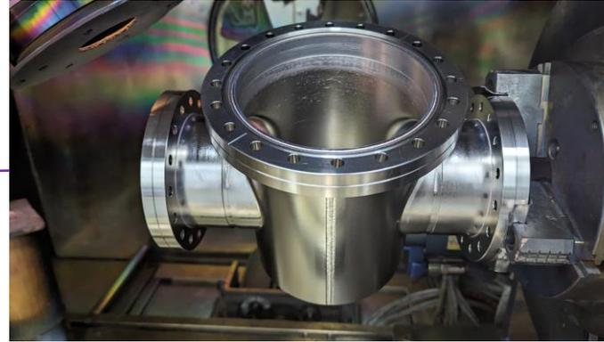
Nb small beampipe with pulled FPC ports
