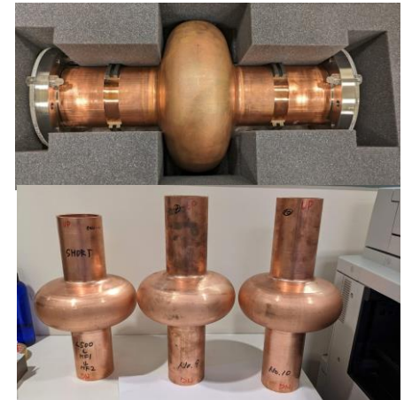
1.3 GHz hydroformed cavities
