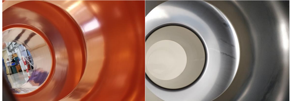
400 MHz cavity before & after coating
