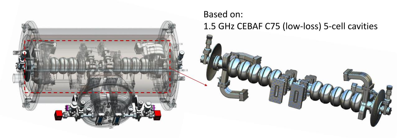
In the framework of G. Eremeev's ECA: "Formation of Superconducting Nb3Sn Phase for Superconducting Radio Frequency (SRF) Cavities"
