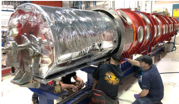
Insertion into vacuum vessel
