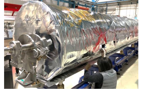
Thermal shield and MLI
