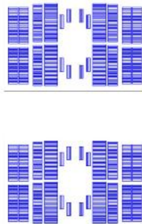
Fig. 1: Main coils of the common coil design (left), main coils (horizontally oriented) with the pole coil.
