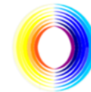
Figure 4.1. Calculated vector field, which indicates the overall current direction for a Roebel cable, shown for an perpendicular uniform applied magnetic field of 0.7T, which was ramped over the virgin curve using a frequency of 0.1 Hz. The operating temperature is set at 4.5 K. The engineering current density of the conductor is scaled to 527 A/mm 2 at 20 T \perp 4.5 K and 4.4 kA/mm 2 at 20 T \parallel 4.5 K in the 100 \mu\text{m} thick tape.
