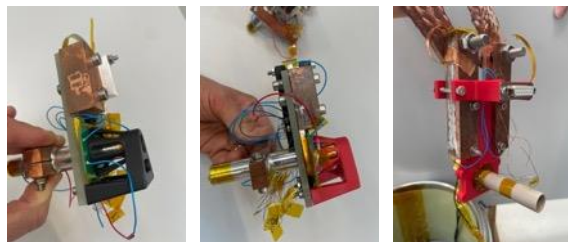
“Baby-HTS” Coils (1-3) with 2-stack single-pancake (1,2) and 1-stack double-pancake (3) geometry.
