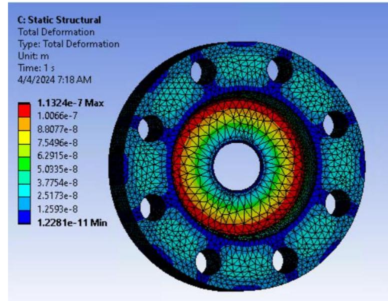
Max deformation  $\approx 0.1 \mu\text{m}$  which is negligible
