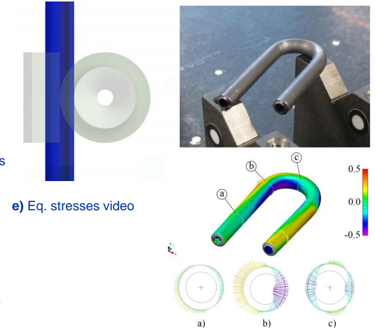
Fig. Step 3. Plastic bending experiment. [T.Coiffet EN-MME CERN]
