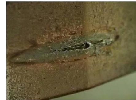
Damage to coated collimator jaw due to accidental beam loss in the SuperKEKB – T. Ishibashi ( talk )
