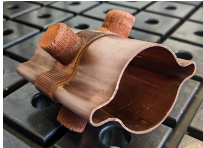
Test of cold sprayed bosses on a chamber prototype
