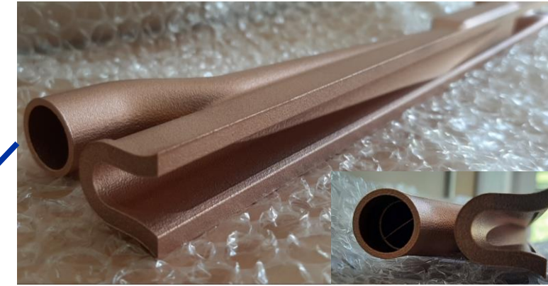
3D printed synchrotron radiation absorber
