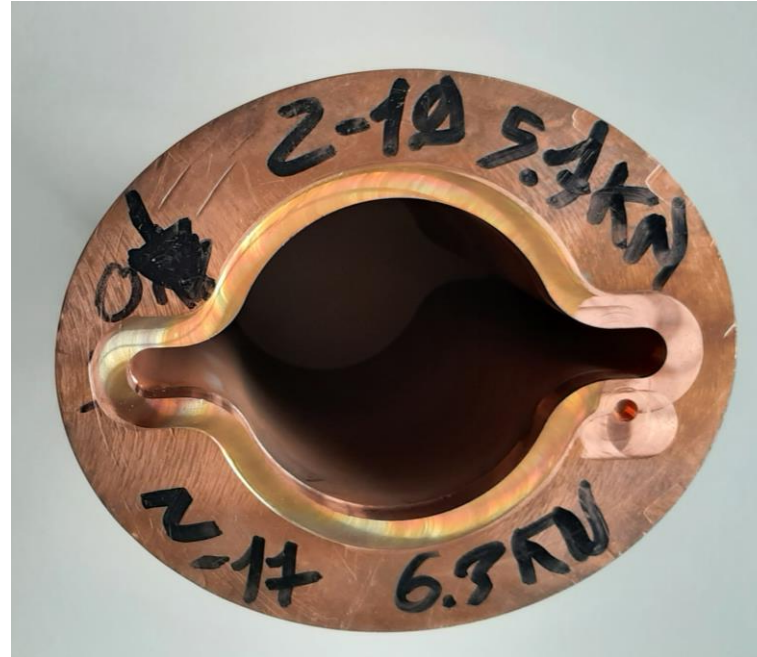
Stir welded flange after local remachining
