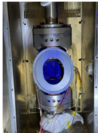
Compact bi-metallic (Cu/St. St.) connection of the BPM pick-up
