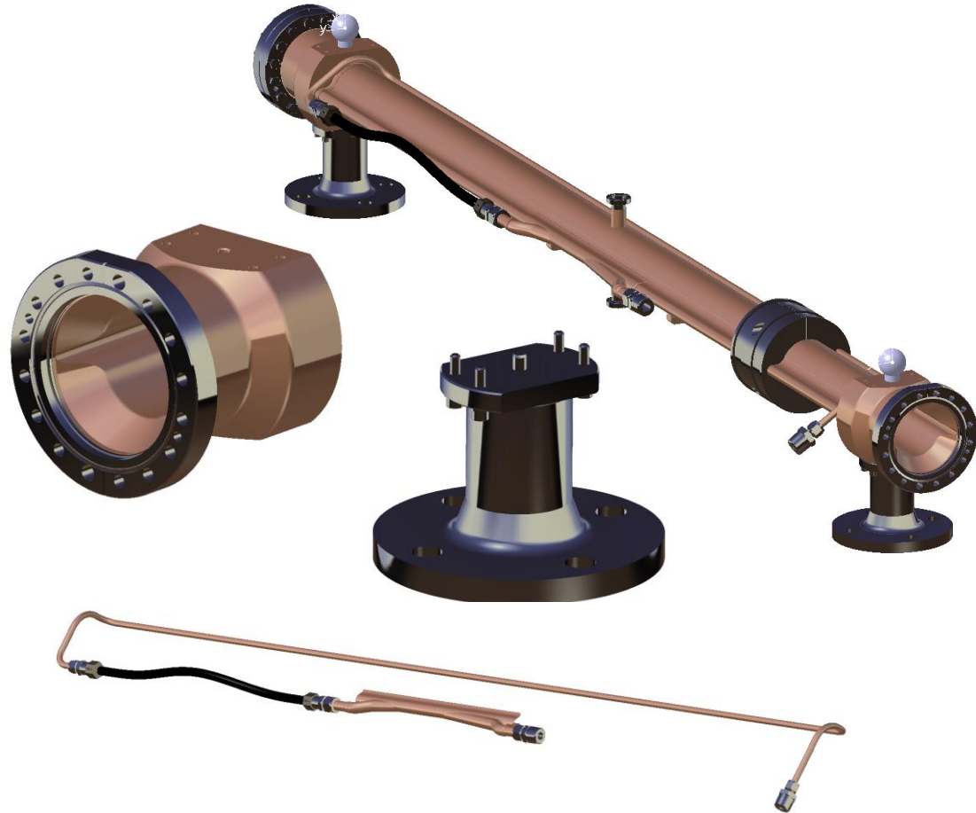
Design of chamber prototype for tests at KARA synchrotron radiation light source
