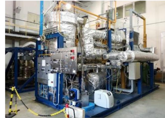
LECOR Corrosion Loop
