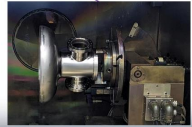
R75mm beampipe welded to half cell
