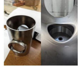
Nb small beampipe with pulled FPC ports
