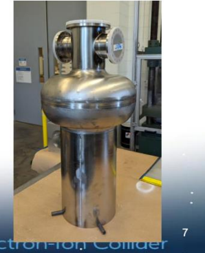
Cavity subassemblies stacked together (some welds pending)
