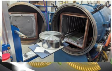
R137mm beampipe stub brazed to a flange
