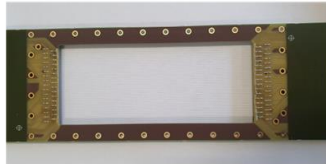
Carbon wire chamber soldered then glued
