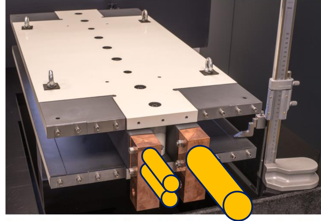
Figure 3.2: One of the ca. 1 m long model dipole magnets manufactured at CERN.
