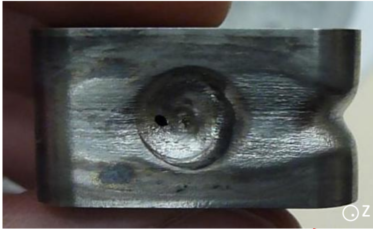
Molybdenum cathode damage
