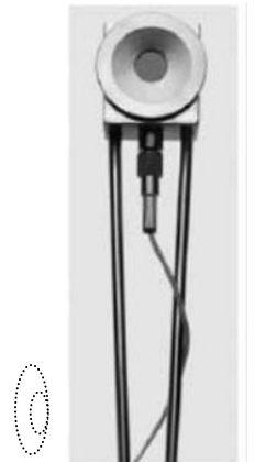
QMB: quartz micro balance; Cs layers are deposited on a quartz detector plate covered by Au.
