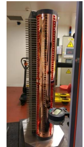
Figures: Precision machined disc (top left), a VNA measurement of an assembled accelerating structure (top right), E-field distribution in a single cell (bottom left). And discs being stacked and aligned prior to bonding (bottom right).
