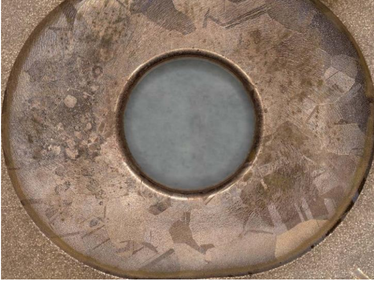
Figure: Images from the post-mortem examination of the CLIC crab cavity [3].
