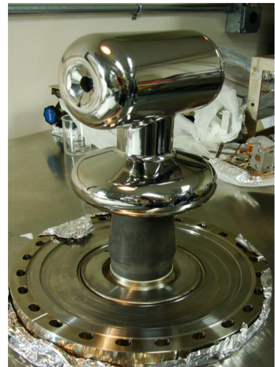
After barrel polishing 60 min. plastic cones 60 min. crushed corn cob
