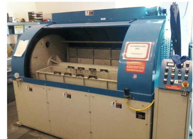
Barrel polishing machine at JLab SRF
