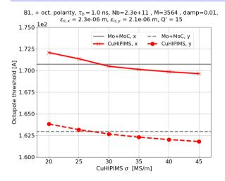
With  $\sigma=$  30 MS/m the threshold is even lower than with Mo+MoC
