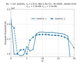
The impedance improvement is mostly in the x-plane, which is the most unstable plane between Q' = 7 and Q' = 20 in the baseline scenario, therefore there are good hopes that the octupole threshold will be improved.
