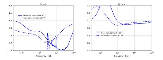
The impedance is significantly improved in the x plane, while in the y-plane the improvement is less significant (but still present around 1 GHz).
