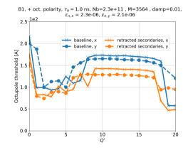
The octupole thresholds are improved by  $\sim$  20%.
