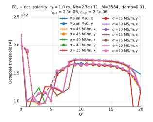
The impact of the material choice on the threshold amounts only to a few amps.
