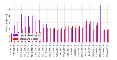
The final re-matched optics for the HL-LHC is not available yet, so this study is carried out by re-matching the HL-LHC optics with the same constraints as the LHC. Even better performance can be achieved in the HL-LHC by relaxing the phase advance constraint.
