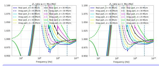
In order to not increase the impedance around 1 GHz with respect to the Mo+MoC case, CuHIPIMS should have a conductivity of at least 30MS/m.
