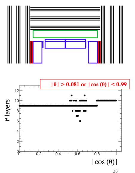
In the transition region from barrel to end cap  $(0.5 < | \cos(\theta) | < 0.8)$  the muon passes sometimes less, sometimes more than 9 layers.
