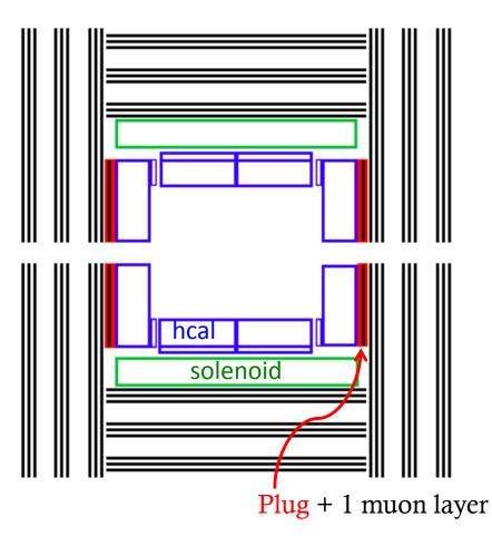
Each endcap includes a plug, with a 10<sup>th</sup> layer. This is to have the magnetized yoke start immediately where the coil ends, improving B-field uniformity.
