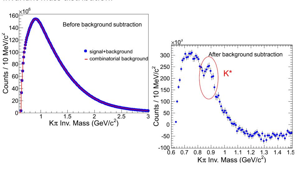
The signal was obtained by subtracting the combinatorial background distribution (through mixed event technique) from the kaon-pion invariant mass distribution.
