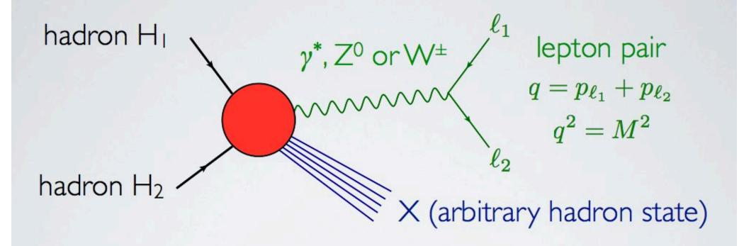
The production of a lepton pair with large invariant mass is the most basic hard-scattering process at a hadron collider.
