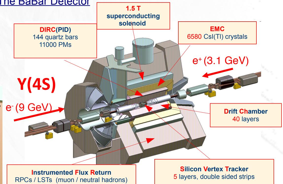
SVT: 97% efficiency,  $15 \mu\text{m}$  z hit resolution (inner layers, perp. tracks)
