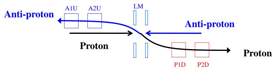
Momentum dispersion in horizontal plane results in more halo (beam background) in the IN/OUT detectors, so concentrate on vertical plane AU-PD and AD-PU to maximize |t| acceptance while minimizing background
