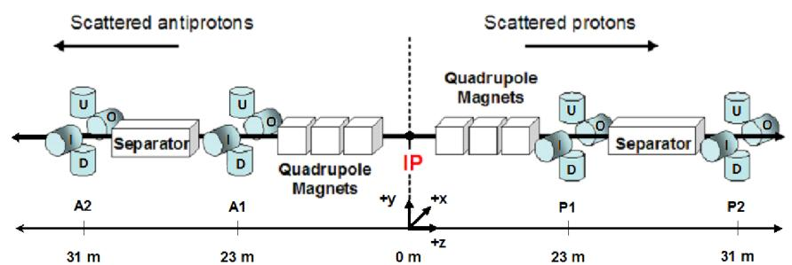
⇒ There are 8 quadrupole spectrometers 4 each (Up, Down, In, Out) on the outgoing proton (P) and anti-proton (A) sides, with each spectrometer comprised of two detectors (1, 2)
