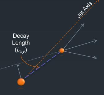
Remaining displaced tracks fit to common vertex Remove the worst tracks
