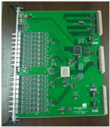
PMT Front End Electronics 1.5625 ns TDC 300 ns ADC shaping
