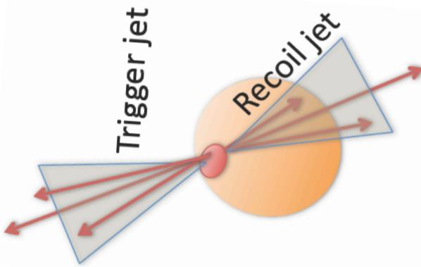
High tower trigger - single particle with high  $p_T$  bias maximizes distance through medium recoil jet traverses
