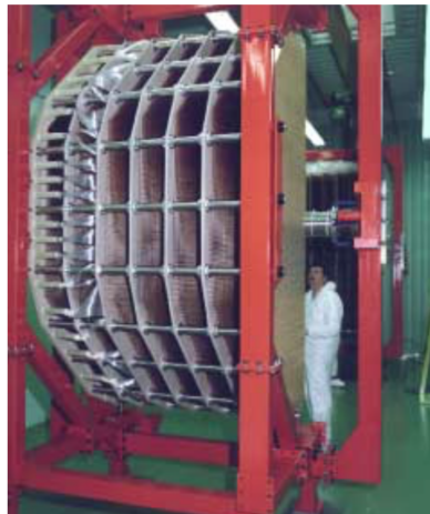
Electrode structure (half) of the Liquid Krypton Calorimeter, now used by NA62, cold ( \sim 120 K) since 1998
