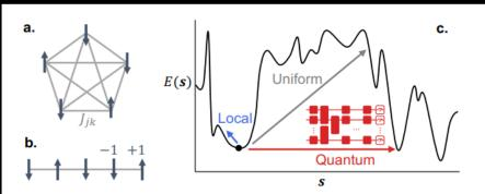
FIG. 1. Ising model representations. a. Graph depicting an n = 5 model instance where arrows (vertices) represent spins and edges represent the  $\binom{n}{2}$  non-zero couplings  $J_{jk}$ . Fields  $h_j$  are not shown. b. An n = 5 model instance with only n - 1 non-zero couplings. c. A rugged energy landscape typical of spin glasses, with the configurations  $s \in \{-1, 1\}^n$ depicted in 1D. Typical proposed jumps for three MCMC algorithms, from a local minimum, are shown for illustration.
