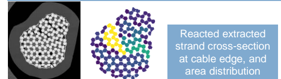
Aspect ratio distribution of well separated \text{Nb}_3\text{Sn} after heat treatment
