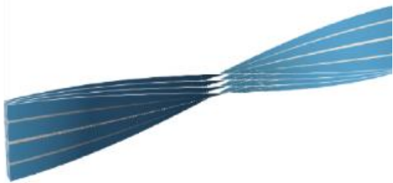
Twisting flat HTS tape
