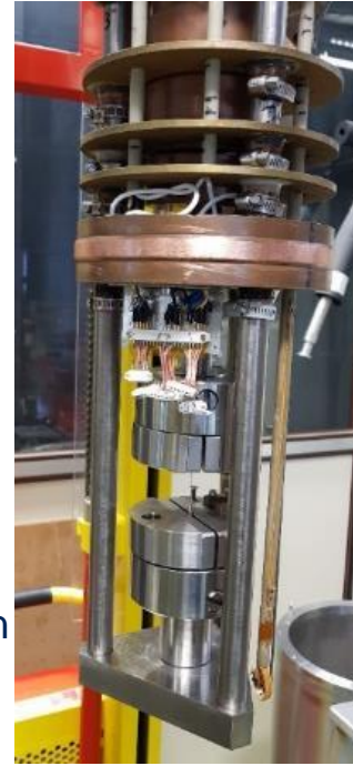
Mechanical characterization of Nb 3 Sn strands at ambient/nitrogen
