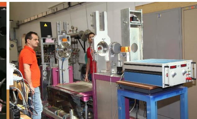
Rotating coil bench
