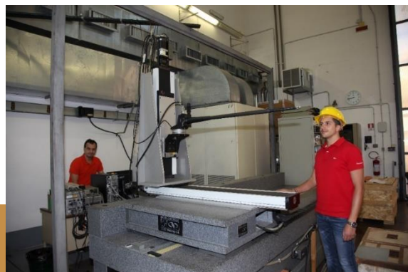
Hall probe mounted on the coordinatometer
