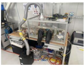
Tensioning table for two reels, based on CERN design. Flux-foamer. Automatic winder unit with pneumatic pushers, heater controls etc. Vacuum-solder vessel.
