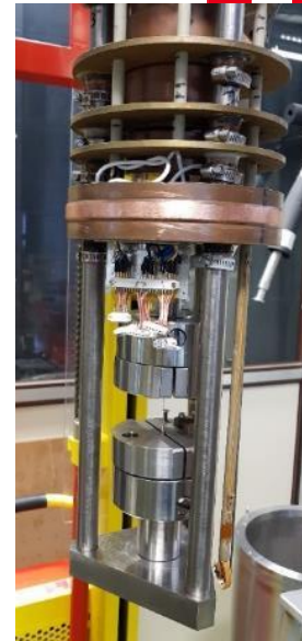
Tensile test of a Nb3Sn strand at 77 K
