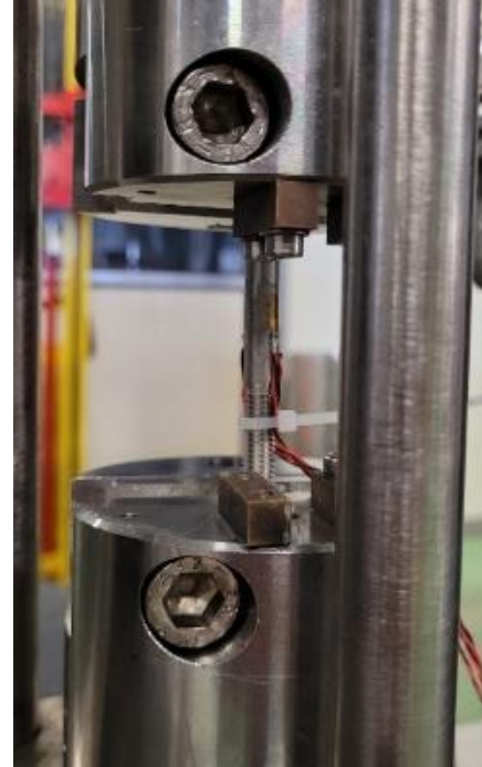
Bolts are being calibrated , pressure homogeneity on the stack need to be evaluate before the first measurement
