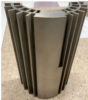
3D printed parts from 316 powder by GE Additive
