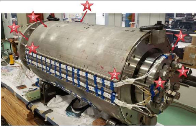
Acoustic sensor locations on shell and rods
