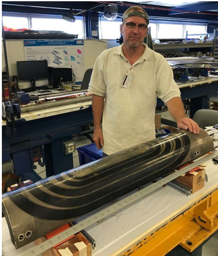
Coil impregnation with epoxy
