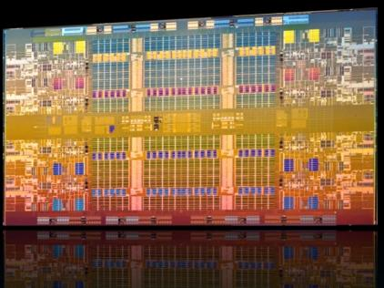
In Intel® MIC architecture, each core is smaller, has lower power limit, has lower single thread performance, but higher aggregate performance Many core relies on a high degree of parallelism to compensate for the lower speed of each individual core
