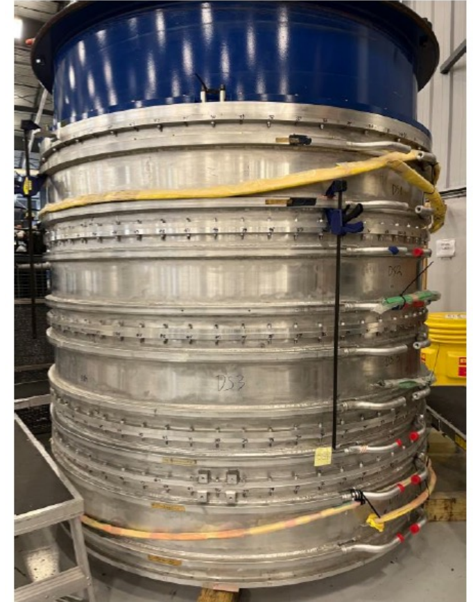
Mini cold mass: coils 1-4 bolted together
