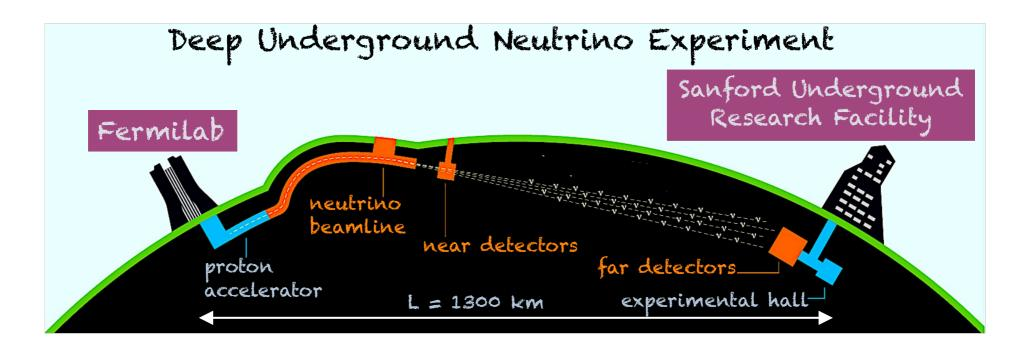
for the first time, a <u>long-baseline</u> (<u>1300 km</u>) <u>oscillation</u> experiment will use argon as its nuclear target for precision studies of V oscillations
