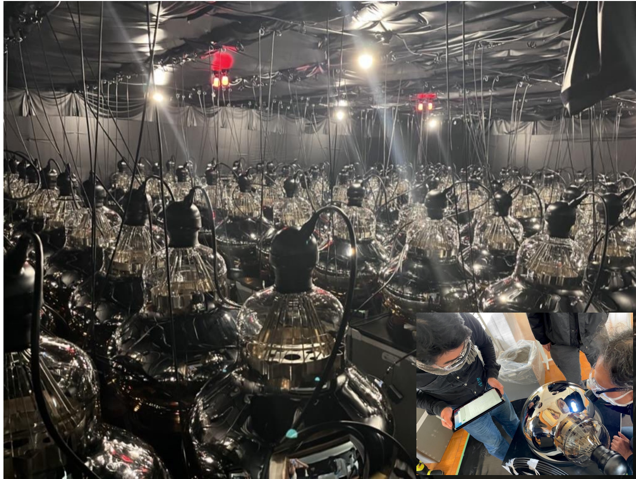
50 cm PMT production ongoing, >6000 already delivered Screening both at Hamamatsu and Kamioka
