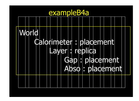
If this is not set, given "Gap" and "Abso" are placed with copy number 0, energy deposition and track length are accumulated for all layers.
