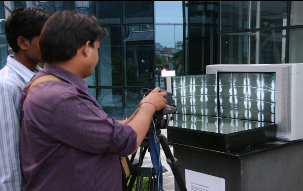
Basic Video-feedback set up. Mirrors at right angles to the TV add to the image complexity and are a way to create iterated function systems of fractals.
