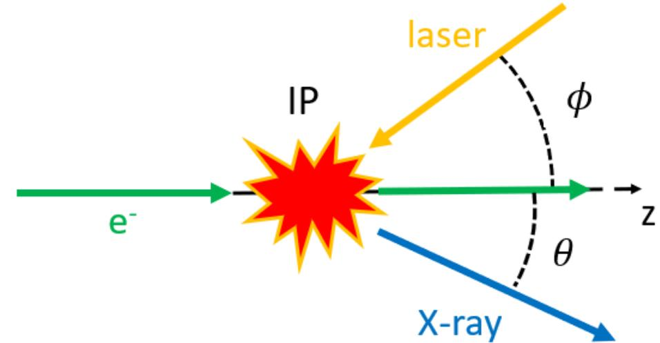
$$N_{\gamma} = \sigma_c \frac{N_e N_{\text{laser}} \cos(\phi/2)}{2\pi\sigma_{\gamma,y} \sqrt{\sigma_{\gamma,x}^2 \cos^2(\phi/2) + \sigma_{\gamma,z}^2 \sin^2(\phi/2)}}$$
