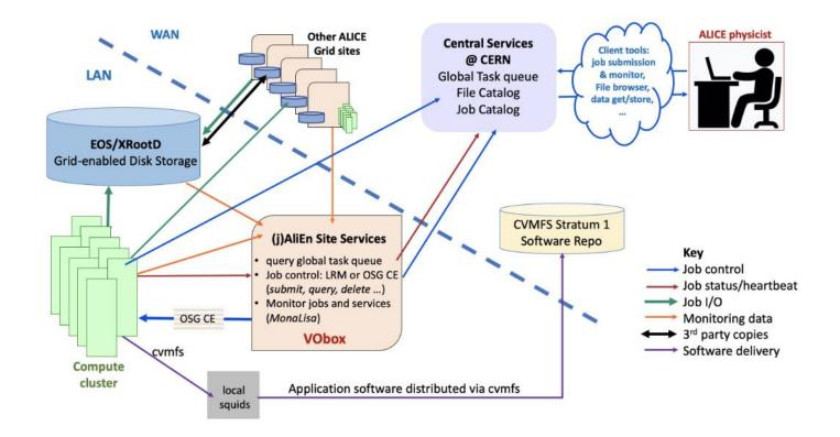
Schematic cartoon of ALICE Grid site internal topology and relative to the larger grid facility.
