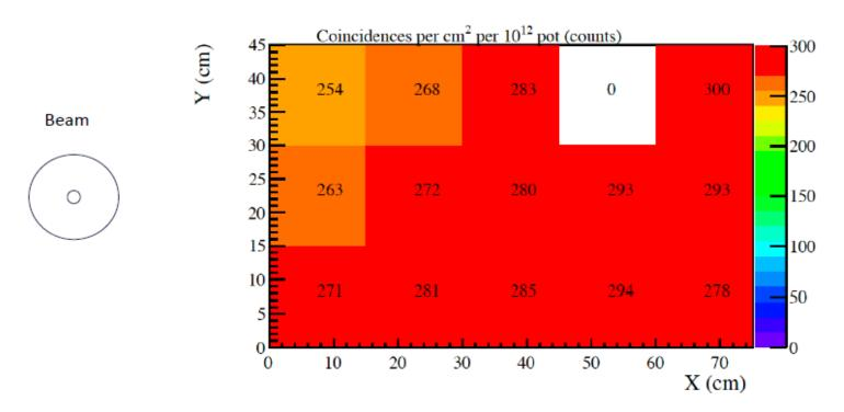
Measured Rate: 250-300 counts/cm2/spill, increasing by increasing the distance from the beam
