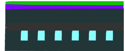
Monolithic CMOS detector with integrated micro-channels
