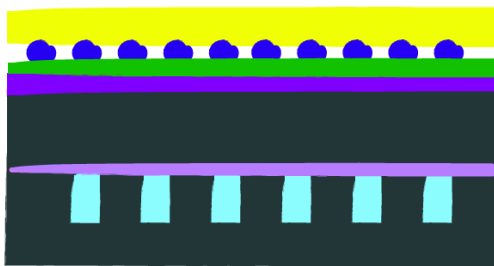
Hybrid pixel detector & micro-channel cooling plate
